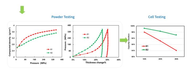
After assembling into half-cells following the same procedure, cycling at 3.0~4.3V, 0.5C, and 45 °C, sample B2 exhibits better cycling stability.
