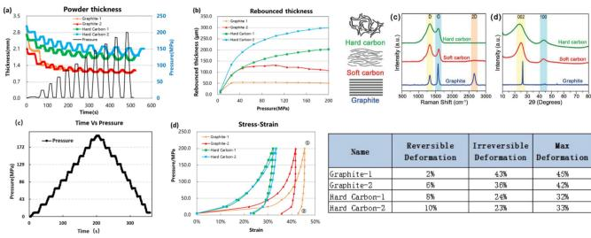
Conclusion: the conductivity of graphite is greater than that of hard carbon, so is its powder compressibility.
