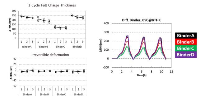
**Conclusion:** The irreversible swelling of the 4 tested cells is similar, and the main difference lies in the **swelling thick-ness after one cycle of full charge**, that cells with **binder C** outperformed the others.
