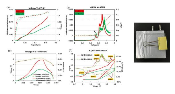
**Test Conditions:** O Pouch Cell(stacking) ⊘ 200 mAh (1 cycle) ⊘ Cathode: NCM811 ⊘ Anode: 450Si/C (450 mAh/g) 800Si/C (800 mAh/g)
