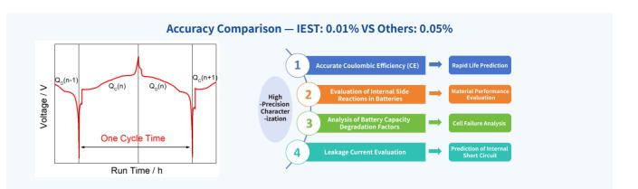
The 0.01% testing accuracy can precisely measure the specific capacity of new materials and detect subtle side reactions during the initial stages of battery cycling. This allows for a comprehensive performance evaluation and lifetime prediction of the battery in a short period.
