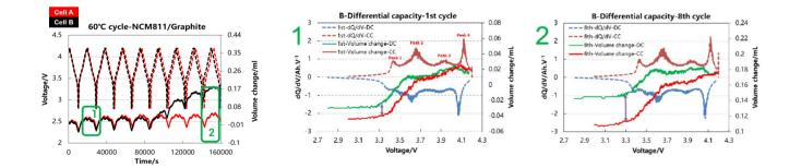
Test Conditions: ⊘ NCM/Gr Pouch Cell ⊘ Temperature: 60°CRate: 0.5C ⊘ Voltage: 3-4.2V
