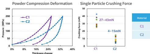
**Conclusion:** The compressive property of particle C1 is stronger. Hence, C1 powder shows a higher compression modulus than that of C2.
