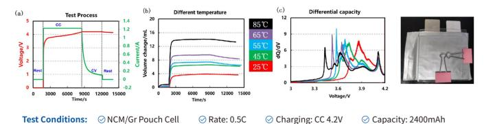
**Conclusion:** The gas production increases gradually with the increases of formation temperature, and when formation temperature is around 55°C, the first phase transition reaction peak will be more acute.
