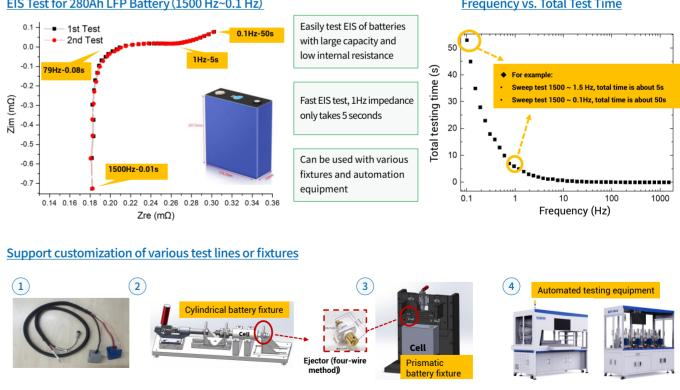
The EIS test frequency range can be adjusted according to the production line progress and process section
