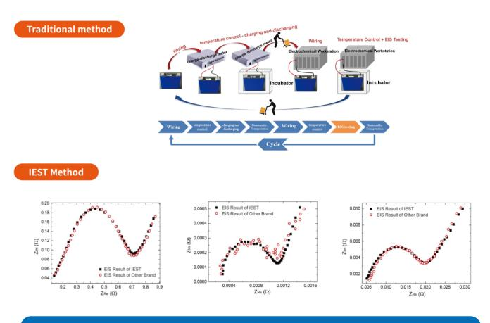
Minimize wiring, handling, and temperature adjustments, streamline operations
