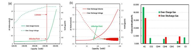
Test Conditions: ⊘ LFP/Graphite Cells ⊘ 0.5C CCCV to 5V ⊘ 0.5C DC to 0V
