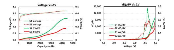
21700 Cell parameters: Sample 1-15%SiC ; Sample 2-10%SiC The volume swelling curve during formation shows that as the silicon content increases, the volume swelling during formation process increases, and the peak corresponding to lithium intercalation on the differential capacity curve becomes higher.
