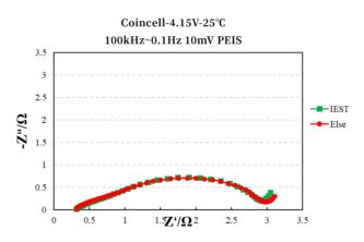
Compared with the EIS test results of well-known foreign electrochemical workstations, the error is within 5%.
