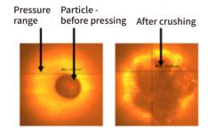
The two NMC materials A1 and A2 are sintered from the same precursor, but the sintering process is different. The particle size D50 is 18 µm.
