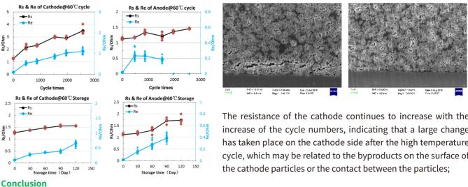
The resistance of the cathode continues to increase with the increase of the cycle numbers, indicating that a large change has taken place on the cathode side after the high temperature cycle, which may be related to the byproducts on the surface of
