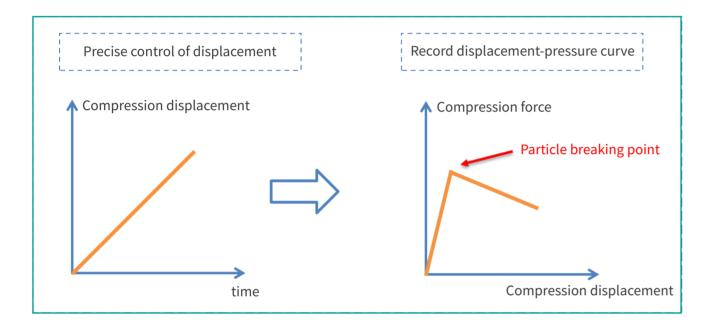
Particle Compression Property and Powder Compaction
