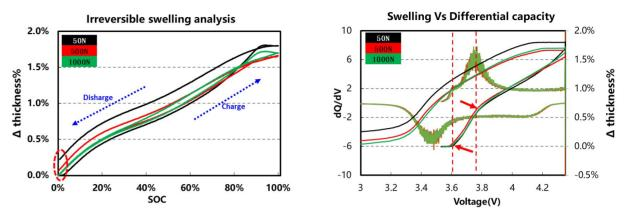
Test Conditions: ⊘NCM523/Gr Prismatic Cells(2400 mAh) ⊘34cm\*46cm\*106cm(T\*W\*L) ⊘Pre-stress: 50N/500N/1000N
