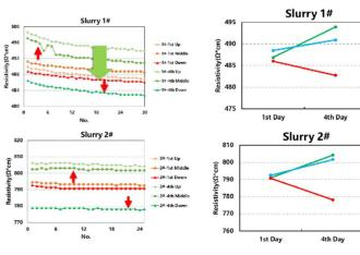
On the first and fourth day of testing, the resistivity of the upper and middle channels increased, while the resistivity of the lower channel decreased, indicating that after four days of shelving, the slurry shows obvious settlement.
