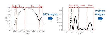
Contact impedance R<sub>4</sub> : The sum of all electronic resistances inside the battery, which is related to various problems Contact impedance R<sub>c</sub>  $\Leftrightarrow$  Area1: problems such as poor soldering of the tab and poor contact SEI film impedance RsEI  $\Leftrightarrow$  Area2: problems such as poor formation folding and wrinkling of the electrode Charge transfer impedance R<sub>a</sub> ⇔ Area3: problems such as poor
