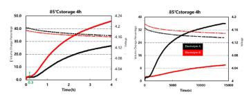
**Test Conditions:** ⊘ 4.2V fullly charged ⊘ storage at 85°C for 4h **Conclusion:** Different cathode materials, electrolytes, and storage temperatures all affect the volume change of the cells.
