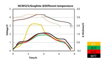
Test Conditions: ⊘ NCM523/Gr Prismatic Cells(2400 mAh) ⊘ Temperature: 0°C/25°C/45°C/60°C
